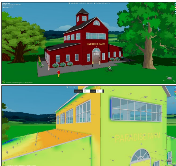
FIGURE 1. An overlay of the daily total solar irradiance (shown as heatmaps) and heat fluxes (shown as arrows) on top of a house (upper) designed in Aladdin.
